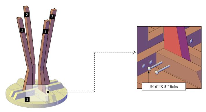
**Step 2:** Turn the table over its feet. After that, attach the Supports-A (3) to the legs with 5/16" x 5" bolts (A) with washers and nuts. Each part has a series of numbers that indicate where to attach the part with the corresponding number.
