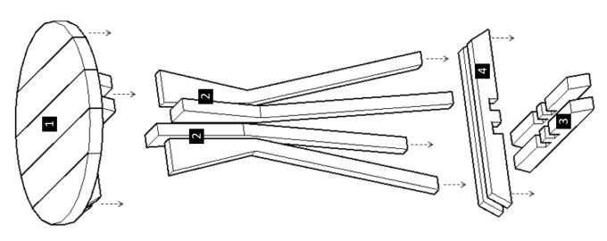
**Step 1:** Place the Tabletop (1) upside down. After that, use 5/16" x 5" bolts (A) with washers and nuts to attach the legs (2) to the tabletop. Each part has a series of numbers that indicate where to attach the part with the corresponding number.
