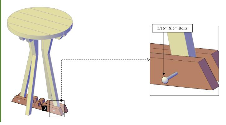
**Step 3:** Finally, use 5/16 ' x 5' Bolts (**A**) with washers and nuts to attach the Supports-B (**4**) to the legs. Each part has a series of numbers that indicate where to attach the part with the corresponding number.
