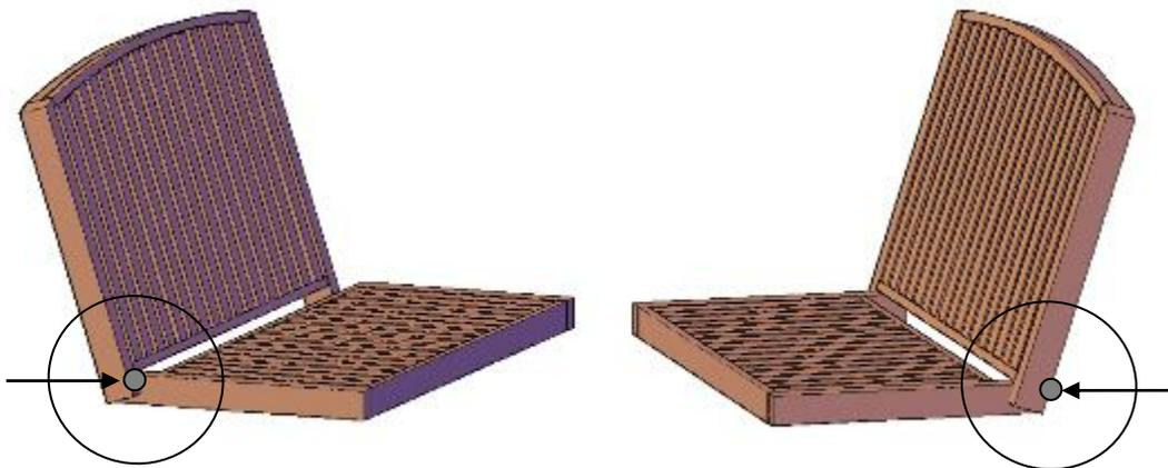
**Step 2:** Attach sides to backrest & seat. Each side has a groove on the inside of the frame for both the seat and the backrest to independently slide within.
