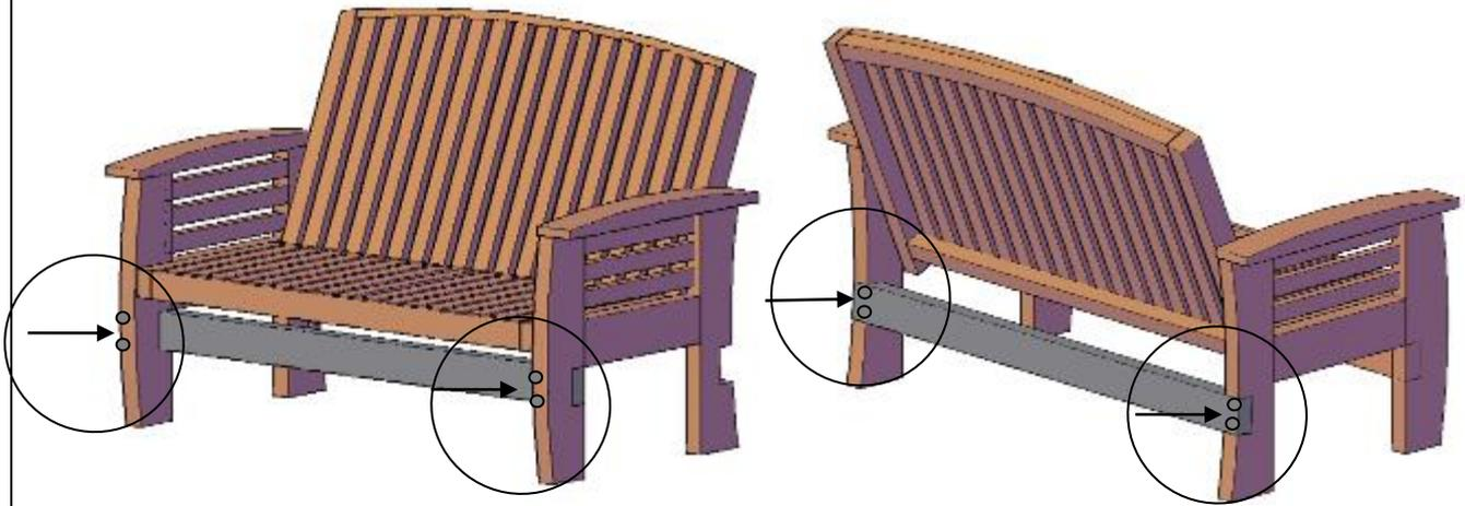
**Step 4:** Attach diagonal support to side and rear support with 2 bolts (3 ½" x 5/16" Bolts), washers and nuts. Match the numbers next to the predrilled holes on the interior of the sides to the numbers on the rear support. Tap the carriage bolts all the way into the wood, then attach the washers, nuts and tighten with ½-inch ratchet. Do not over-tighten. Repeat this step for the other diagonal support.
