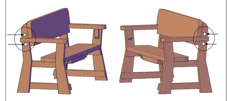
**Step 3**: Attach diagonal supports to seat and sides with 2 carriage bolts (3  $\frac{1}{2}$ " x 5/16), washers and nuts per support.
