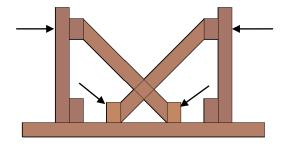
Tiny Benches – Could be 32" or less. 2 deck screws to attach each diagonal support to bench top and one carriage bolt to attach each diagonal support to each leg
