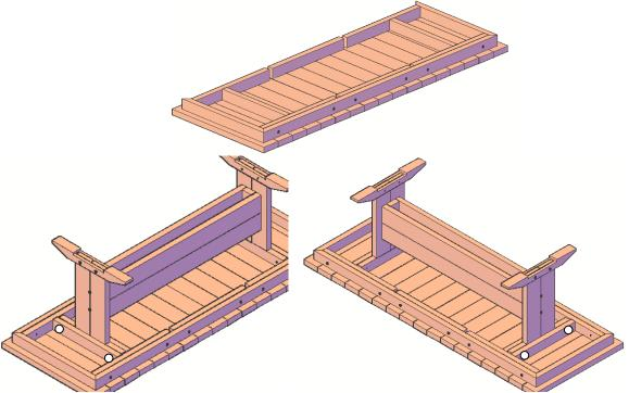
Carefully turn the table around. Be careful not to place all the weight of the table on one leg – the table is very heavy and can damage the point where the leg attaches if too much stress is placed on that point.
