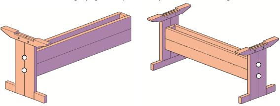
**Step 2:** Place the tabletop on a soft surface upside down. Attach legs to tabletop, with two bolts (4" x 5/16"), washers & nuts per side. Tap the bolt all the way into the wood to set it. Then add a washer and nut and lightly tighten. Make sure the numbers written on both pieces match.
